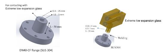
FP cavity valve (2) has to be contacted with metal flange DN40-CF (SUS304) (Sr. No 5) by Vender or by their contacting service provider as per given above diagram.
